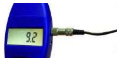
Fig. 10: Connecting the cable to the Wöhler HBF 420
