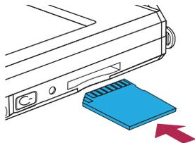
※ Insert the memory card according to the direction.
