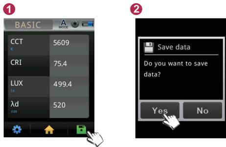
Press Save key on the lower right of the screen, and select "Yes" key.
