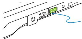
※ When the power is on, the Power button will turn on the green indicator. When the power is off, the green indicator will be off.
