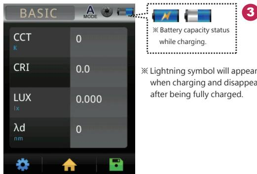
※ Lightning symbol will appear when charging and disappear after being fully charged.
