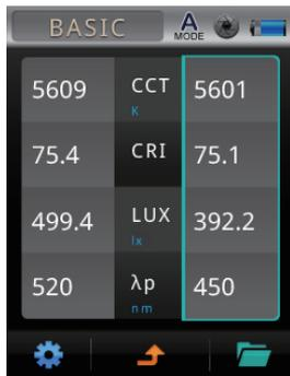
After the measurement is completed, the measured light source data are compared by parallel display.
