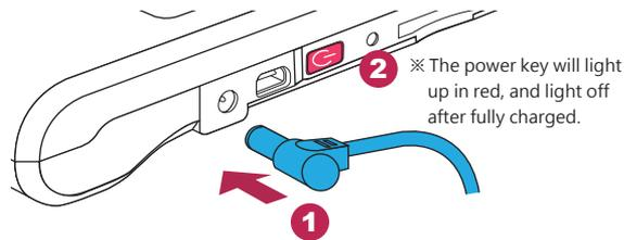
※ The power key will light up in red, and light off after fully charged.
