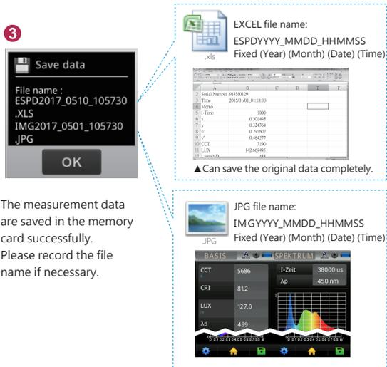
The measurement data are saved in the memory card successfully. Please record the file name if necessary.
