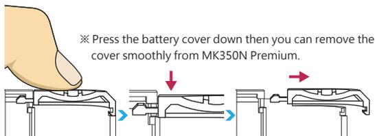
※ Press the battery cover down then you can remove the cover smoothly from MK350N Premium.
