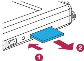
※ Press to remove the SD card
